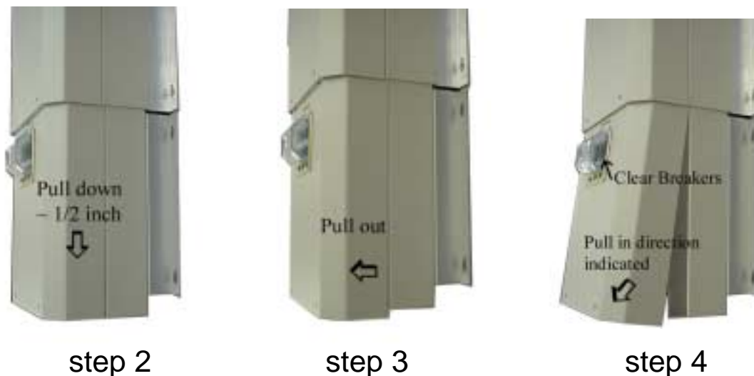
Figure 5. Bottom Cover Removal (Steps 2-4)
